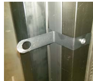
View of bracket installed on Habco cooler
